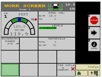
The ISO6 Intelliag system is the latest 8-channel control system from Dickey-john. Based on the ISO-11783 standard, the system is plug & play through any compatible terminal, allowing use of documentation, section control, prescription maps & boundary shutoff. Virtual section switches enabled via an unlock, available through the primary module.
