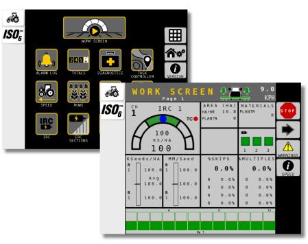
The ISO6 Intelliag system is the latest ISOBUS Rate Controller from Dickey-john. The system supports up to 48 rows of Individual Row Control, ensuring accurate seeding rates across the entire bar, even while turning, using Row by Row Turn Compensation.
