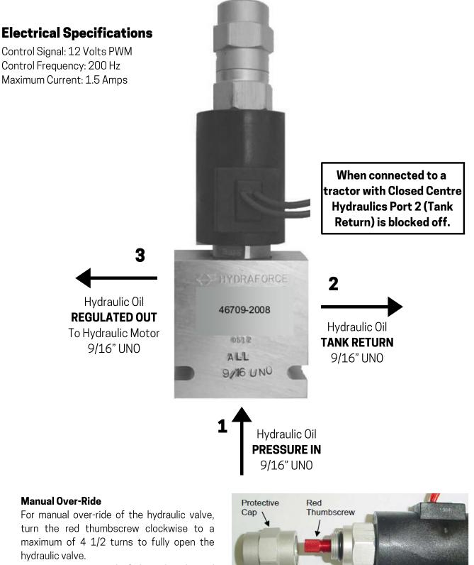
For automatic control of the valve the red thumbscrew MUST be turned fully anticlockwise until it stops turning.
