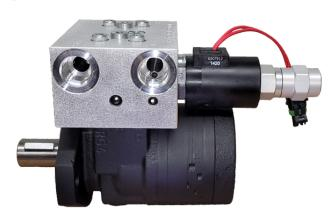
This hydraulic drive delivers high torque at low speeds while consuming very little hydraulic oil. You can gang HydraDrives together using the hydraulic ports provided on the drives. You no longer need chains and sprockets to reduce RPM, the HydraDrive can be connected directly to the final drive shaft. Because the HydraDrive has been designed to work with closed centre hydraulics, you don't bypass unused hydraulic oil, which means more hydraulic oil is available for other operations.
