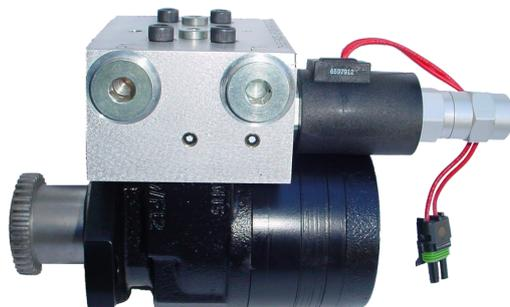
This hydraulic drive delivers high torque at low speeds while consuming very little hydraulic oil. You can gang HydraDrives together using the hydraulic ports provided on the drives. You no longer need chains and sprockets to reduce RPM, the HydraDrive can be connected directly to the final drive shaft. Because the HydraDrive has been designed to work with closed centre hydraulics, you don't bypass unused hydraulic oil, which means more hydraulic oil is available for other operations.
