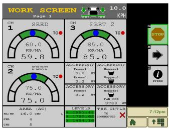
The ISO6 Intelliag system is the latest 8-channel control system from Dickey-john. Based on the ISO-11783 standard, the system is plug & play through any compatible terminal, allowing use of documentation, section control, prescription maps & boundary shutoff. Various unlocks give the user features like virtual section switches & implement folding; all through the base module.
