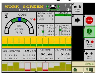
The ISO6 Intelliag system is the latest 8-channel control system from Dickey-john. Based on the ISO-11783 standard, the system is plug & play through any compatible terminal, allowing use of documentation, section control, prescription maps & boundary shutoff. Various unlocks give the user features like virtual section switches & singulation; all through the base module.
