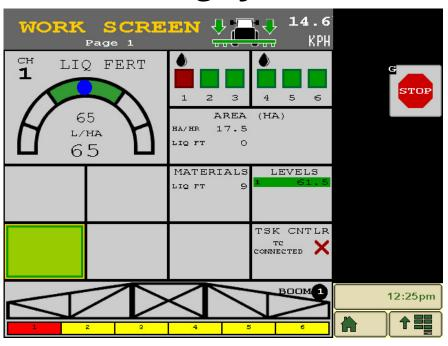
The ISO6 Intelliag system is the latest 8-channel control system from Dickey-john.
